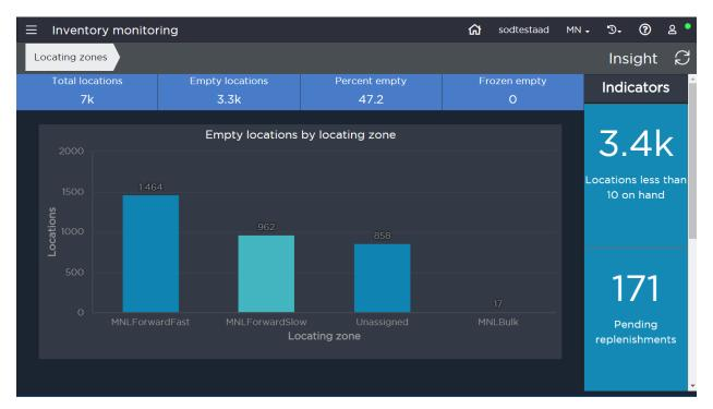
The inventory monitoring screen shown here, like many within Manhattan SCALE, also includes a Pane on the right side of the screen that contains Live Tiles. Selecting either the graph components or items in the surrounding Panes will take the user to a filtered Insights screen of those specific real-time details.
